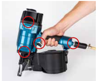
Check for air loss and leaks
