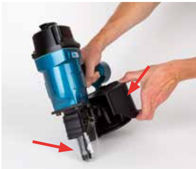
Inspection of the protective and magazine covers
